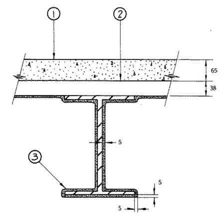
Beam — Beam-W200x36, Minimum Size.
